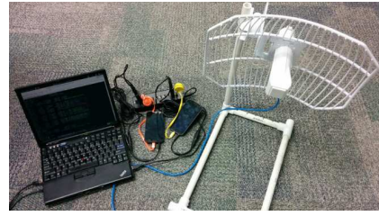
Fig. 6: PhoneHome remote node equipment. The remote node includes a PC, GSM devices to bridge traffic onto a nearby commercial carrier, and a long-distance Wi-Fi antenna to connect to the local node within the camp.
