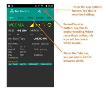
Figure 3: A screenshot of the NetMonitor Cell Signal Logging app, along with tutorial directions taken from the operations manual.
